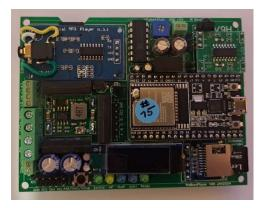
sensitivity/speed of the incoming pulse signal. The on-board processor can be programmed through a micro-USB connector (or updated over-the-air). Stand-alone, the board is powered through the external 24VAC and converts this to 5V through the on-board voltage converter. The board is 7.5 cm x 9 cm and can be mounted in a 3W100, 3WA/160, DEC, Consolette or other popular wallboxes, or outside in a separate housing.
